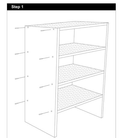
Assemble by attaching all shelves with Screws using # Phillips screwdriver.
